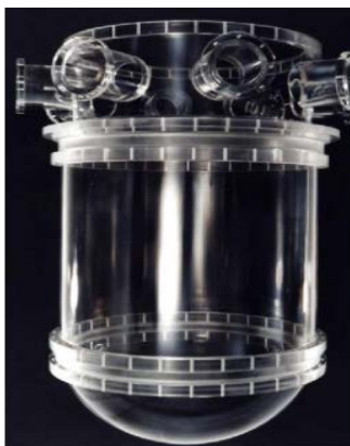
Fig.1. Perspex model of the RPV in ROCOM (IAEA-TECDOC-1908, 2020).
