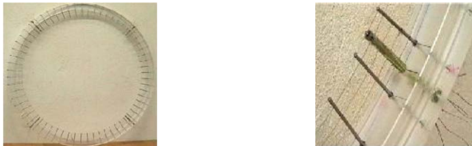
Fig.4. Wire mesh sensor in the downcomer for radial measurements (64x4 measuring positions) (Puragliesi, 2020; Höhne et al., 2006).
