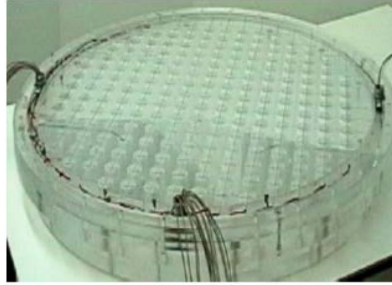
Fig.5. Wire-mesh sensor in the core inlet plane(Kliem et al., 2008; Höhne et al., 2006) .
